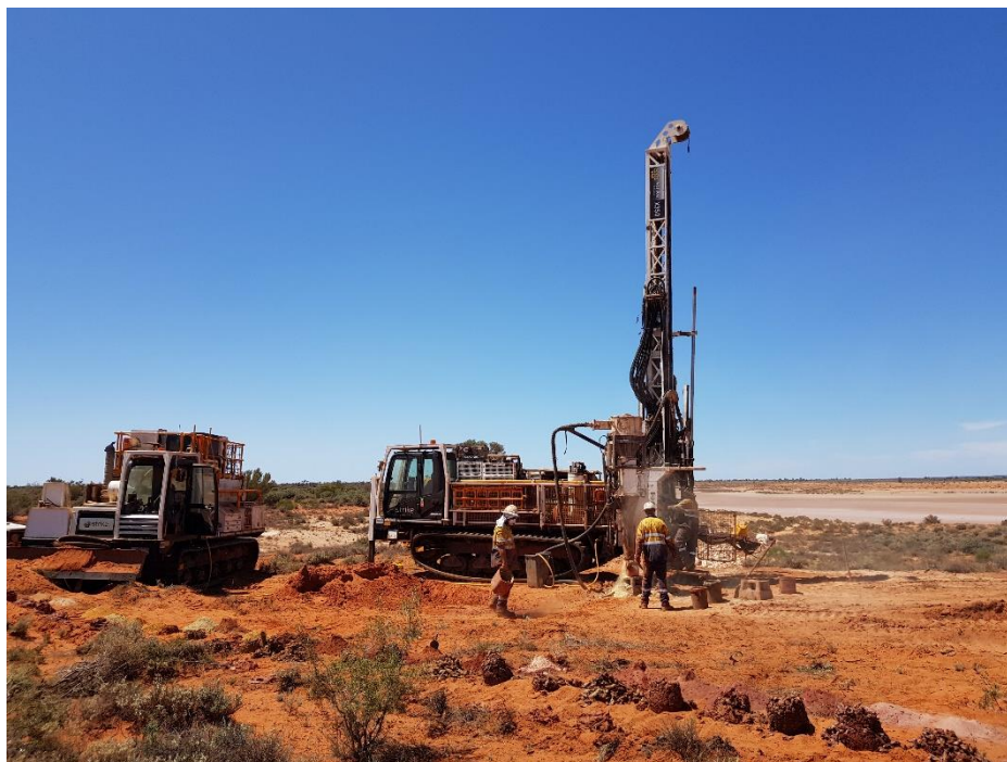
Figure 3: Track Mounted Aircore Rig at FF1
