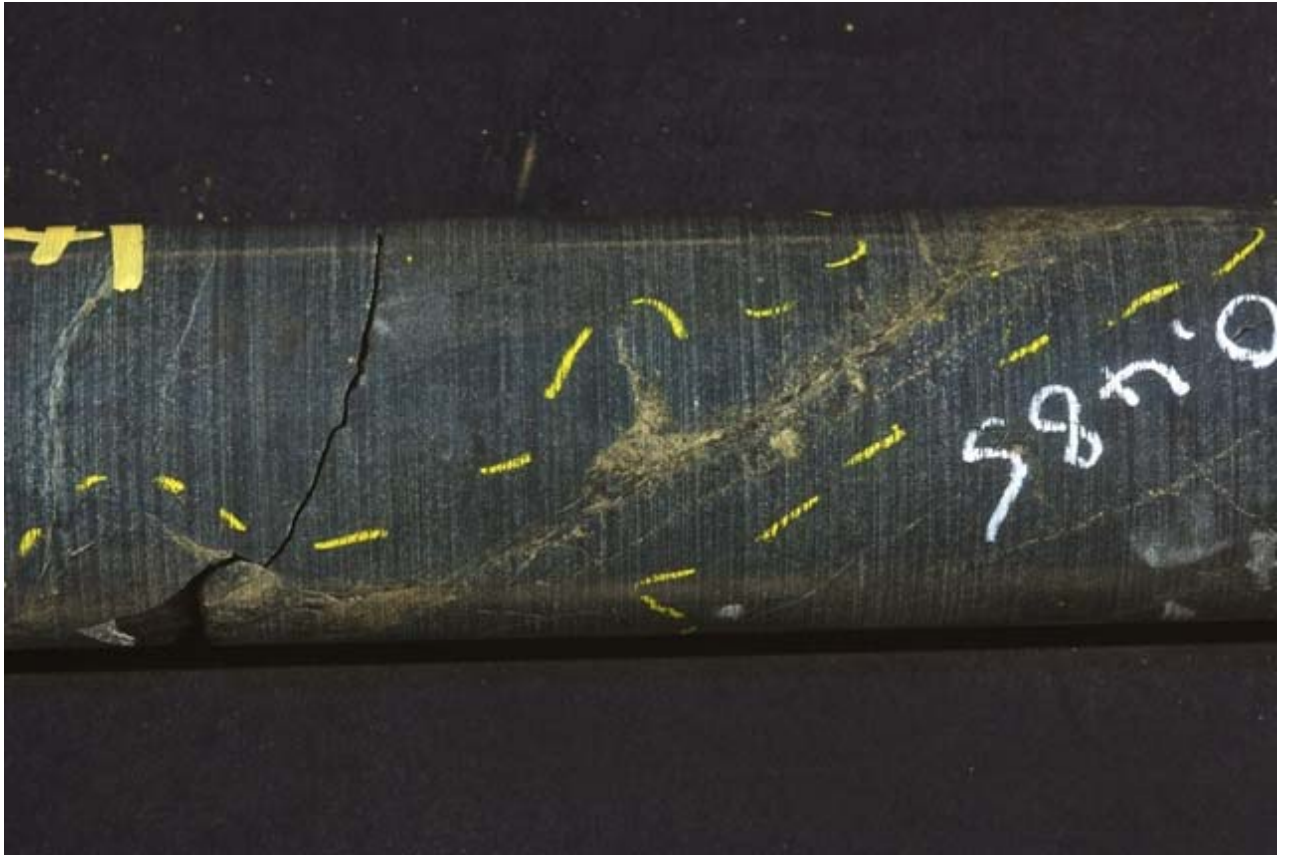
Photo Plate 1: Nickel bearing sulphide vein from CDH05.
